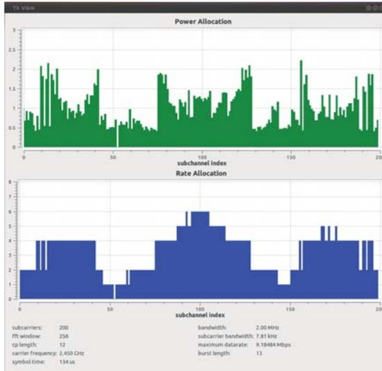
Figure 8.14.: The transmitter's GUI.
