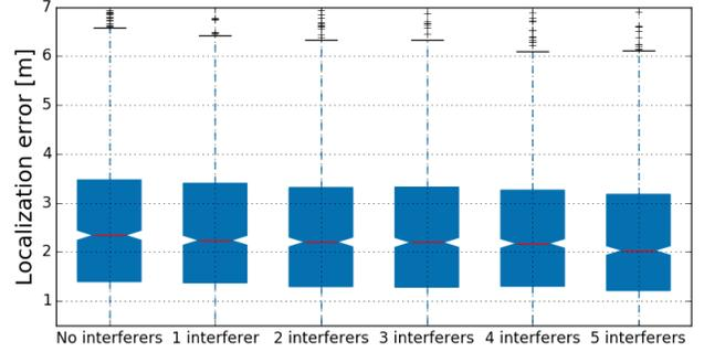
Fig. 7: Influence of the number of interferers in both phases of fingerprinting on the localization accuracy
