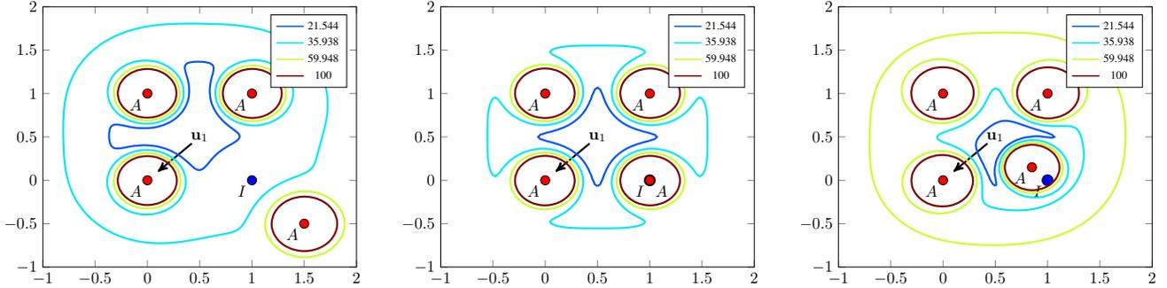
Fig. 4: Effect of anchor placement on  $\ell_{\mathbf{u}_1}(\mathbf{u})$ ; anchors placed as  $(0.5 + \delta, 0.5 - \delta)$  for  $\delta = 1, 0.5, 0.35$
