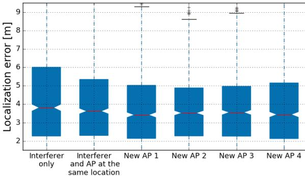
Fig. 10: Performance in a particular area vs. location of an additional AP in relation to interferer's location
