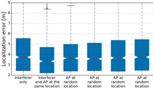
Fig. 9: System level performance vs. location of an additional AP in relation to interferer's location
