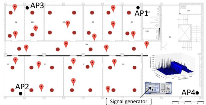
Fig. 11: Locations of APs, training points, evaluation points, and interferer in the testbed environment
