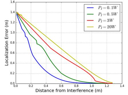
Fig. 2: Localization error versus distance from interference source for different interference powers
