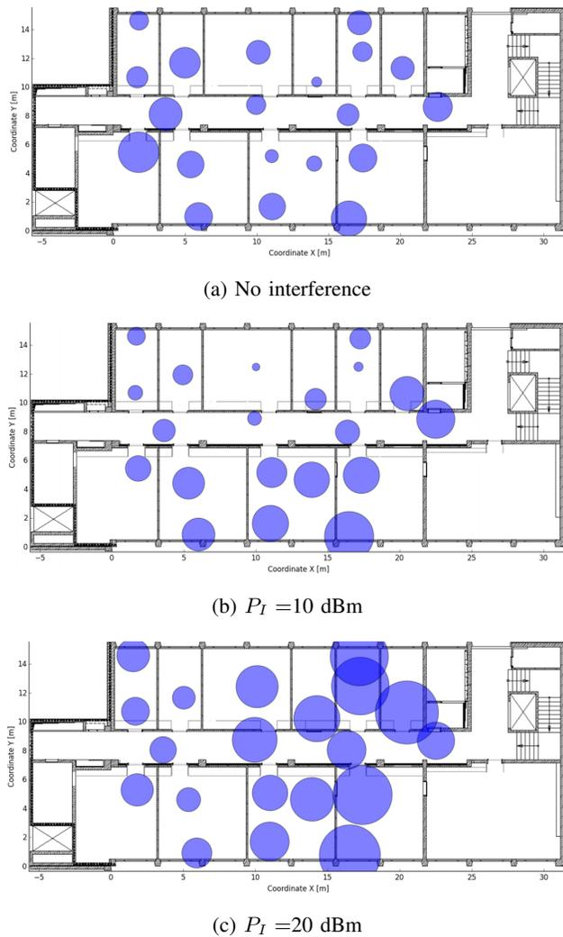
Fig. 12: Spatial distribution of localization errors in the testbed environment
