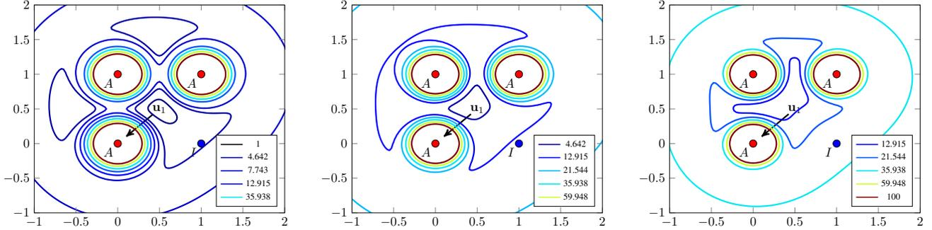
Fig. 3: Identification function for  $\mathbf{u}_1$ ,  $\ell_{\mathbf{u}_1}(\mathbf{u})$  for interference power  $P_I = 0, 0.5$  and  $1 W$  in  $3 \times 3m^2$
