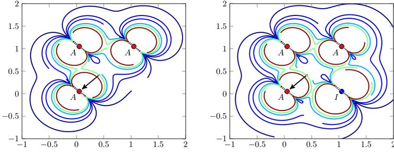
Fig. 1: Resolvability of points with distance 0.14m with 3 anchors (A) and 1 interference source (I) in  $3 \times 3m^2$  - The arrow points toward increasing resolvability.
