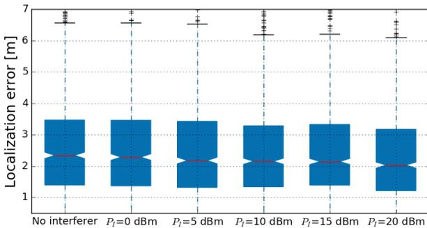
Fig. 6: Influence of the interferer’s transmit power in both phases of fingerprinting on the localization accuracy
