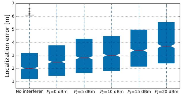
Fig. 8: Influence of the interferer’s power in the measurement phase of fingerprinting on the localization accuracy
