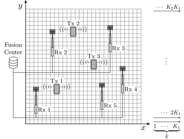
Figure 1. A sensing scenario with  $M = 3$  signal sources  $\text{Tx}_m$  and  $N = 5$  sensing nodes  $\text{Rx}_n$  connected via a backhaul to the fusion center.
