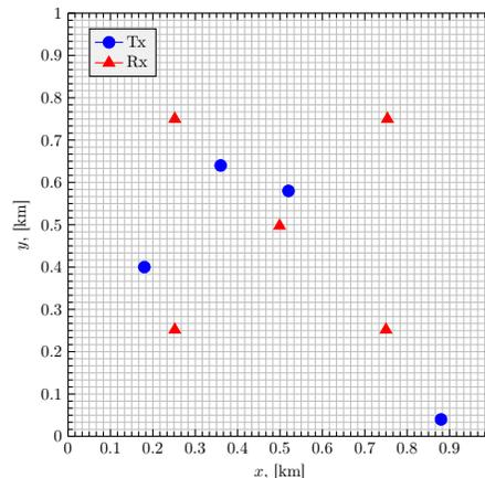
Figure 2. A single realization of a sensing scenario for numerical evaluation with  $M = 4$  signal sources  $\text{Tx}_m$  positioned randomly and  $N = 5$  sensing nodes  $\text{Rx}_n$  located at coordinates  $x_n^r, y_n^r \in \{0.25, 0.5, 0.75\}$  km.
