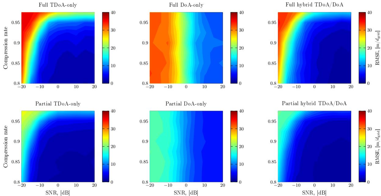
Figure 3. RMSE vs. SNR vs. compression rate for 3 considered scenarios and two recovery approaches. The first row shows the results for the simultaneous recovery where  $L_j = L$ , whereas the second row presents corresponding figures for reduced-size approach with partial recovery with  $L_j \in [3, 5]$  and fusion.
