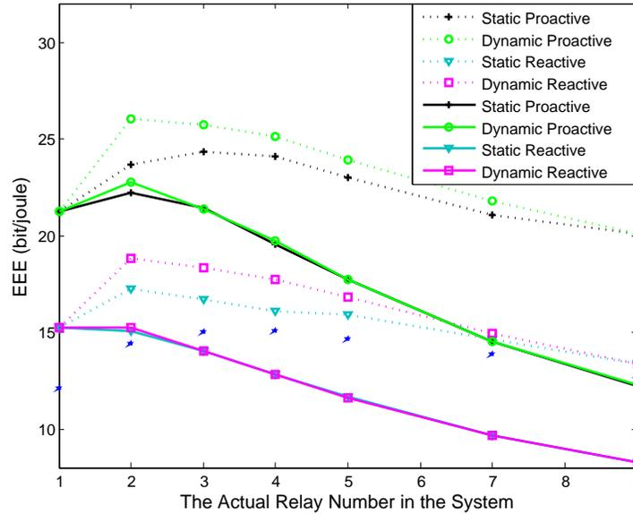
Fig. 10. EEE Performance Loss due to relay number uncertainty.
