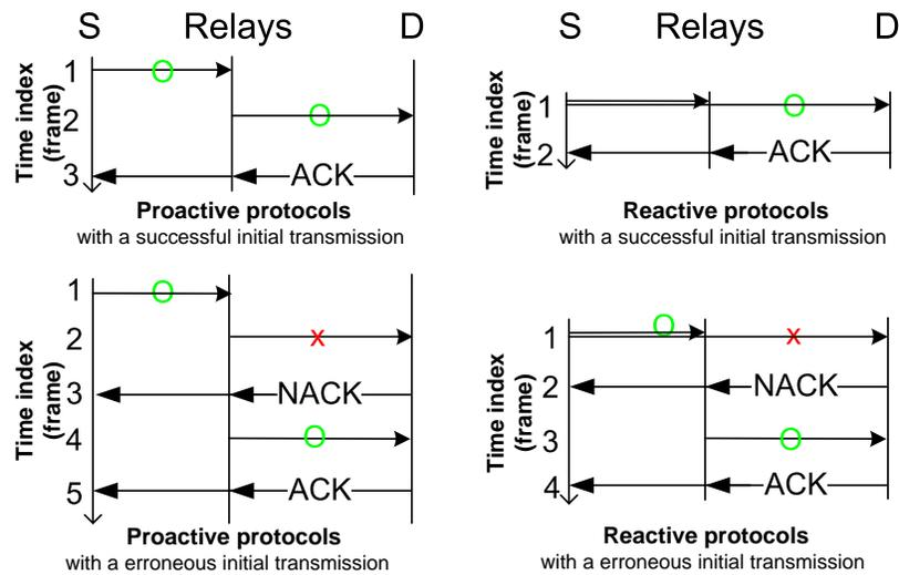
Fig. 2. The difference between proactive protocols and reactive protocols.
