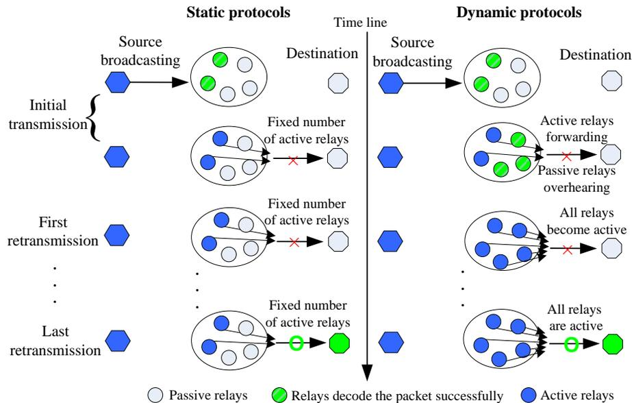
Fig. 3. The difference between static protocols and dynamic protocols.
