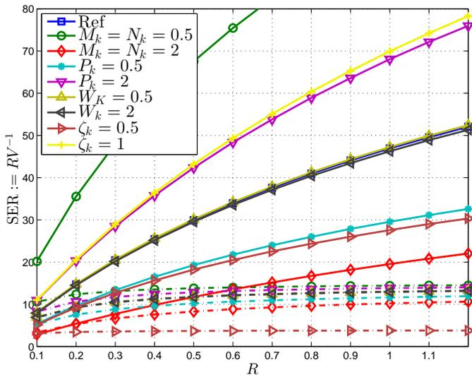
Fig. 4: Reference signal to error power ratio vs. target signal power ( $R$ ). A SN failure-aware design becomes more critical for bigger values of  $R$ .
