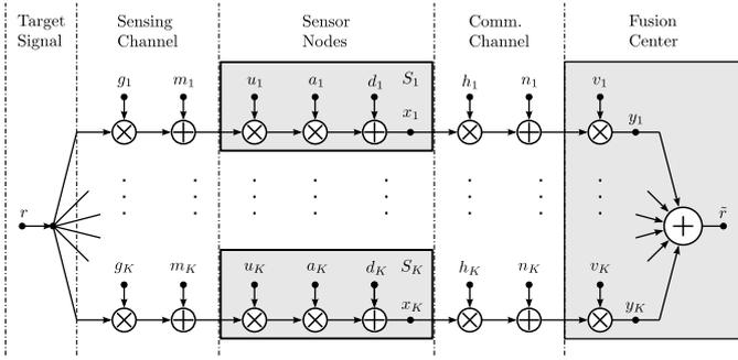
Fig. 1: Signal flow at the defined sensor network consisting of a target signal,  $K$  sensor nodes ( $S_1 \cdots S_K$ ), and a fusion center.  $b_k$  and  $d_k$  describe the possible faulty sensor behavior, see Table I. Detailed explanation is given in Section II.
