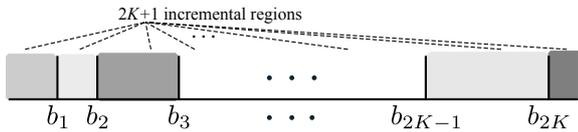
Fig. 2: We obtain  $2K + 1$  incremental regions in order to search for the value of water-level, i.e.,  $\lambda^*$ , where  $b_1 \leq \dots \leq b_{2K} \leftarrow \text{sort}\{J_k(0), J_k(U_k/c_k), \forall k \in \mathbb{F}_K\}$ .
