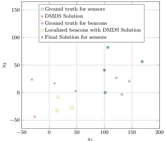
Fig. 2: The steps of the self-localization and anchoring process visualized. The final solution is obtain using Procrustes analysis on the localized beacons.
