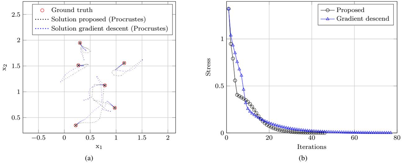
Fig. 3: Trajectories of the sensor nodes during the iterations of the algorithm (a), together with the Stress functions (b).
