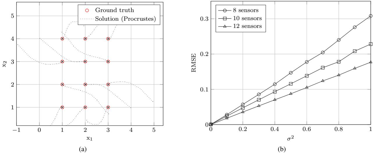
Fig. 4: A simple scenario to study the behavior with noisy measurements (a). Adding more sensors and thereby more measurements, results in improved robustness of the self-localization against the measurement noise (b).
