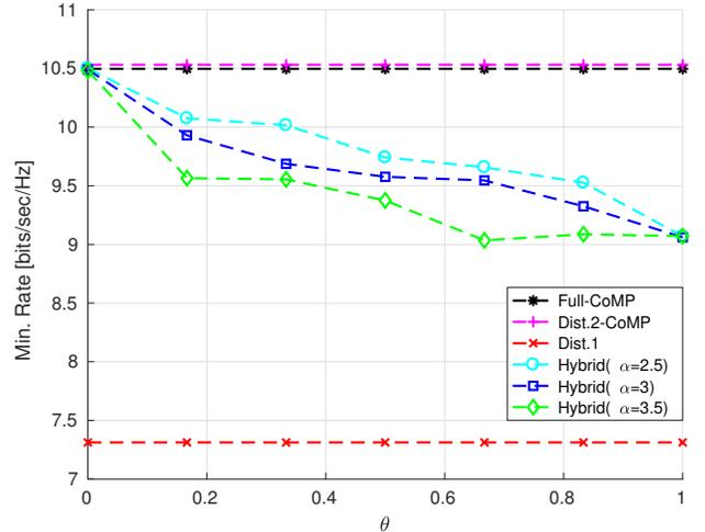
Fig. 2. Min. User Rate vs. Cooperation Threshold. Less cooperation reduces the minimum user rate performance, as cell edge users suffer.
