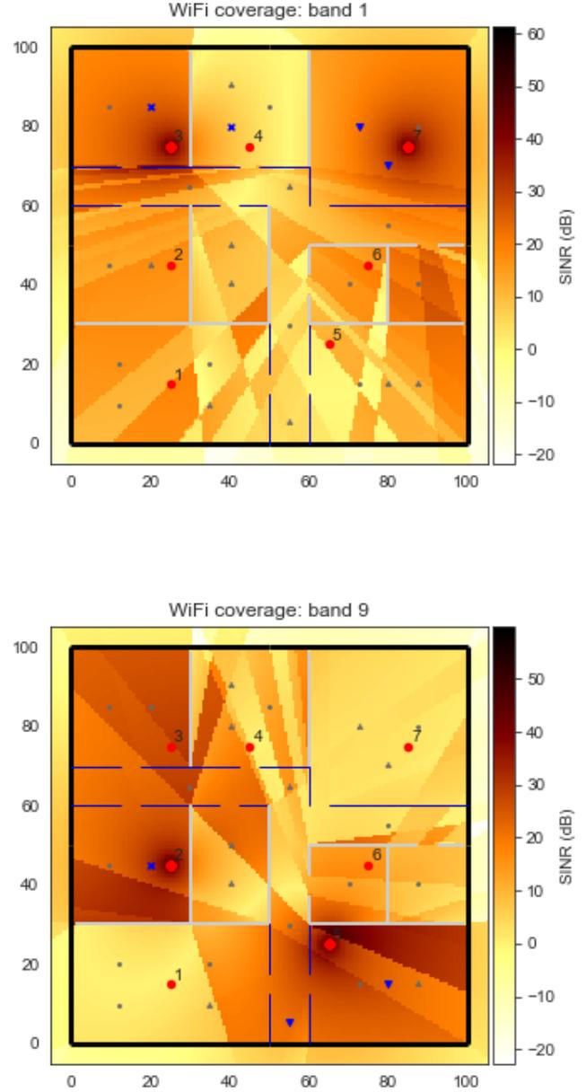
Fig. 1. Simulation results for WLAN network, channels 1 and 9. Deployed access points denoted by red circles, demand nodes by grey circles and triangles for LTE and WLAN, respectively. Top figure: access points 3 and 7 are deployed at WLAN channel 1 and assigned to blue crosses and triangles, respectively. Bottom figure: access points 2 and 5 are deployed at WLAN channel 9, and assigned to blue cross and triangles, respectively.
