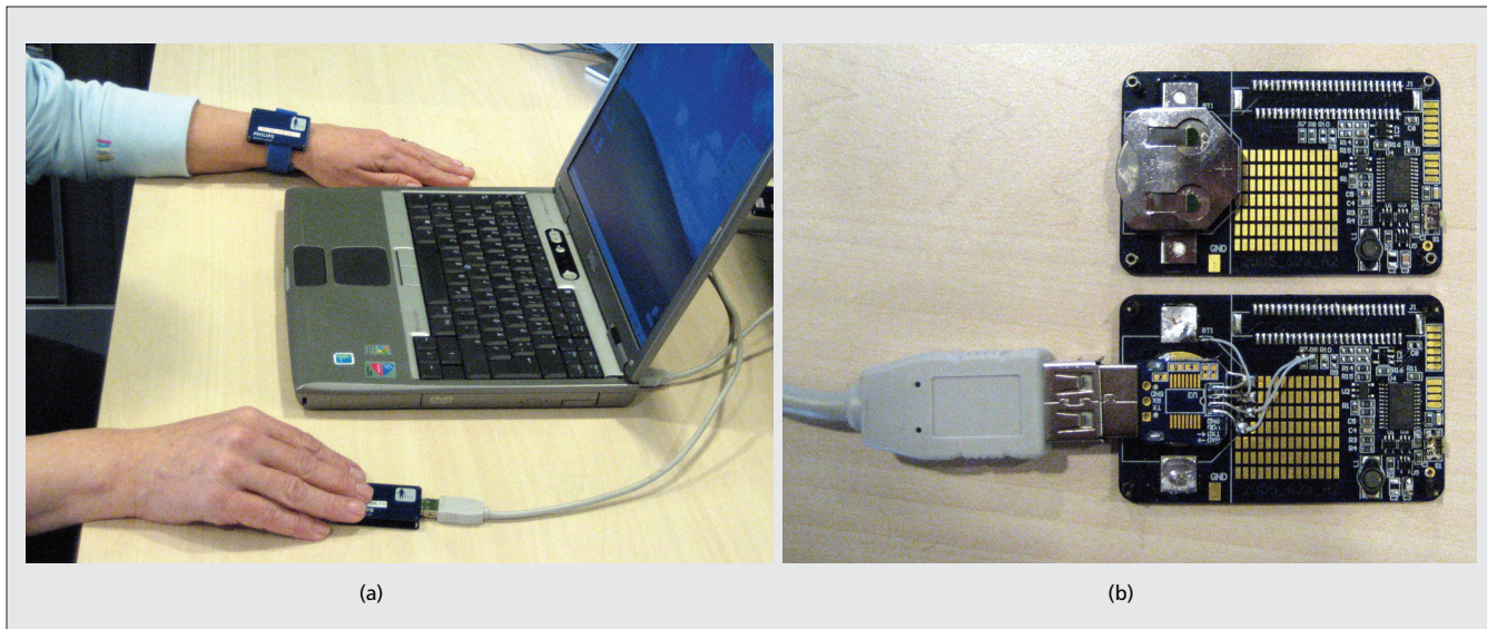
Figure 3. A user identification application using BCC: a) identification setup for user authentication on a laptop using a BCC identification tag on the user's wrist and a USB connected BCC transceiver; b) inside of the BCC transceivers with 3 cm × 5 cm electrodes. The upper transceiver, as worn at the wrist in a), is battery fed. The lower device additionally implements a USB connection, which is also used as power supply.
