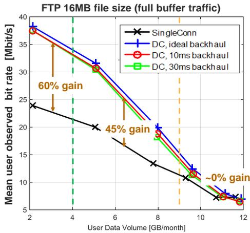
**Figure 5** Average user observed bit rate and gains for 16 MB FTP file transfers
