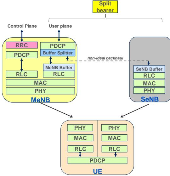
**Figure 2** Dual Connectivity split bearer architecture
