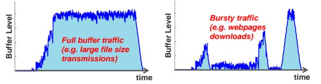
**Figure 3** Buffering of Packets at the eNB
