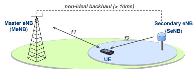
Figure 1 LTE Dual Connectivity (DC)
