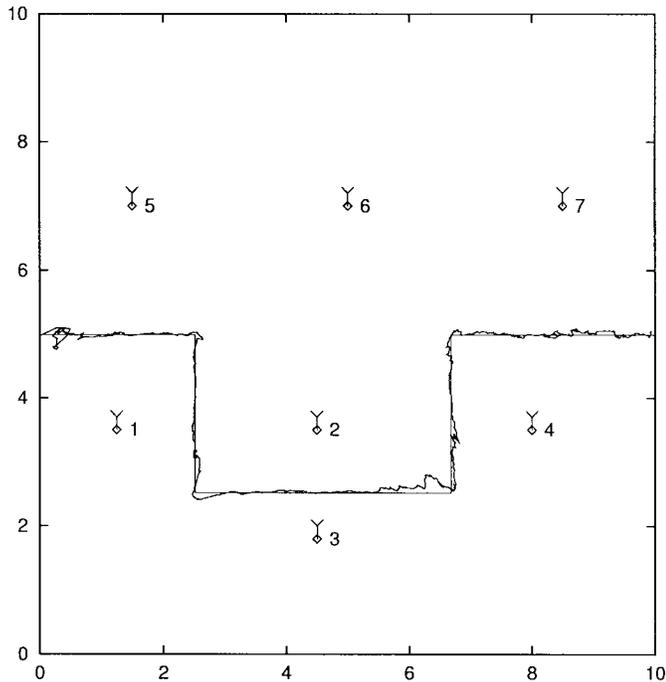
Fig. 3. Estimated track after Kalman filtering.
