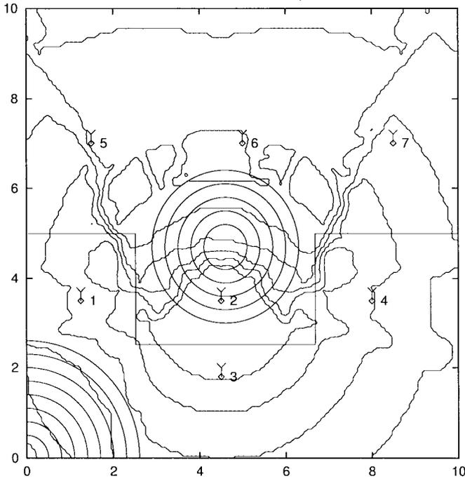
Fig. 1. Base stations, the mobile's track, and isoclines of base station 2.
